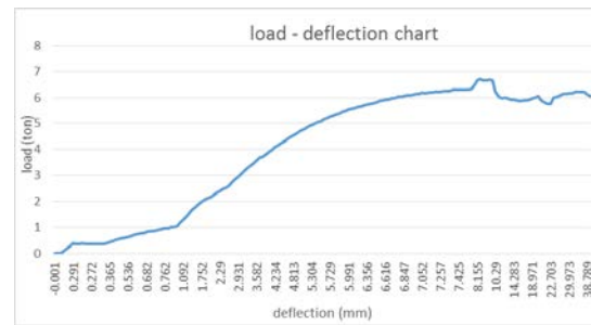
Fig (31) :load-deflection curve of B2
