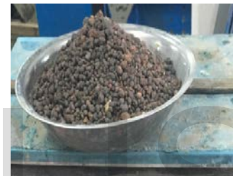
Fig (9): lightweight expanded clay aggregate
